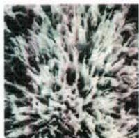
Slag and fly ash blended cement samples were treated with Xypex Admix and examined for evidence of crystalline growth at ages ranging from 8 months to 2 years. Samples were sliced and/or split and examined at magnifications between 500x
